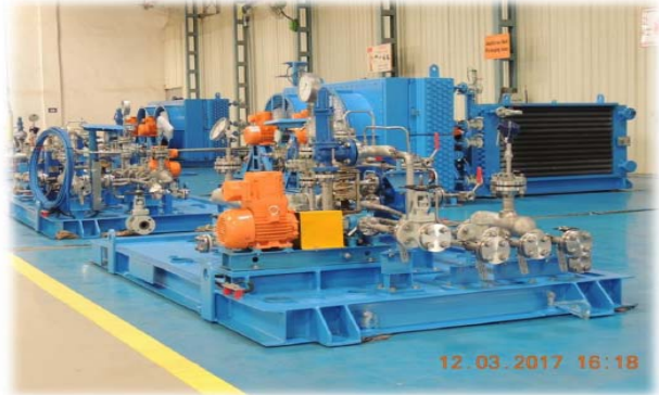
Cooling Lube Oil Console Package Client - ILAM Project, Iran End User- Burckhardt Compression
