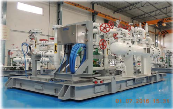
Cooling Water Console Package Client - Rapid Petronas Malaysia End User- Burckhardt Compression
